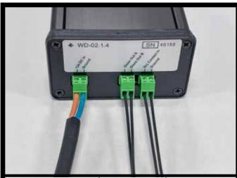
**Step 6** — Connect the power supply to a 120VAC power outlet. **Confirm** system is working correctly.
