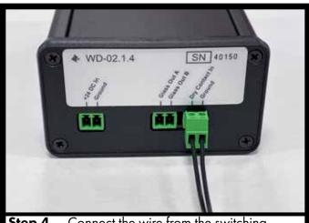
**Step 4** — Connect the wire from the switching mechanism or automation system to the "Dry Contact In" and "Ground" terminals on the controller.
