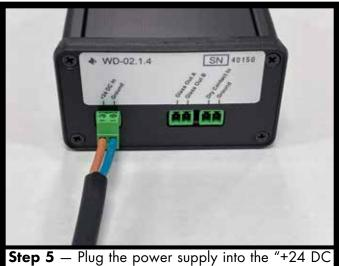
**Step 5** — Plug the power supply into the "+24 DC In" and "Ground" terminals.
