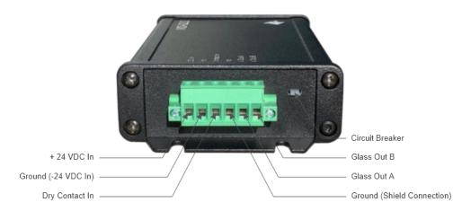
**Note:** Shielded wire must be used for all connections to the WD-02.2. The shield shall be terminated on the WD-02.2 end of the wire only and shall be connected to either of the 'Ground' terminals as labeled above. The shield at the CLiC Glass end and the Switching Device end can be cut where the cable jacket is removed.
